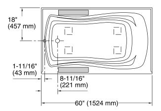
No change in measurements if connected with drain illustrated. (K-7161-AF)
