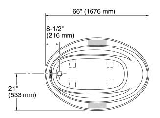
No change in measurements if connected with drain illustrated. (K-37382) Recommended faucet area
