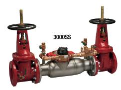
Series 3000SS Double Check Detector Assemblies are designed for use in accordance with water utility non-health hazard containment requirements. It is mandatory to prevent the reverse flow of fire protection system substances, i.e., glycerin wetting agents, stagnant water and water of non-potable quality from being pumped or siphoned into the potable water supply.
