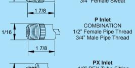
15/16 1/2" PEX Tube Fitting PX3 INLET 3/4" PEX Tube Fitting
