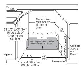
• The rough cabinet opening must be at least 24" deep, 24" wide and approximately 32-1/2" to 34-3/4" high from floor to underside of the countertop.
