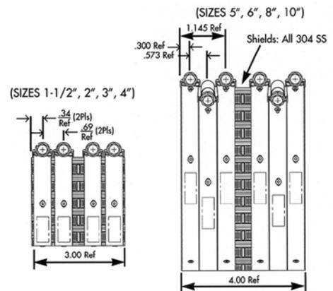
**DESCRIPTION:** Couplings consist of gasket and shield assemblies. The shield assemblies have four or six clamps depending on size. The clamps are fastened with eyelets to the bi-directional corrugated shield.
