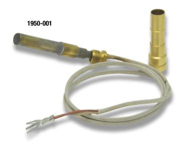
Robertshaw® thermopiles are the industry leader for gas appliance applications. Their primary function is to ensure a standing pilot light is operative so that on a call for heat, the main burner gas will be properly ignited. Thermopiles are placed in gas applications to detect the existence of a flame for safety purposes by shutting off the potential gas flow to a burner.
