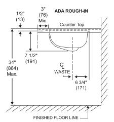
Dimensions may vary (+) or (-) 1/8". Dimensions shown in parentheses are in millimeters: 25.4 mm = 1 inch. Note: Fixture dimensions are nominal and conform with dimension and performance requirements of ASME/ANSI Standards A112.19.4M. Dimensions subject to change or cancellation without notice. Briggs is not responsible for the use of superseded or voided specification information.
